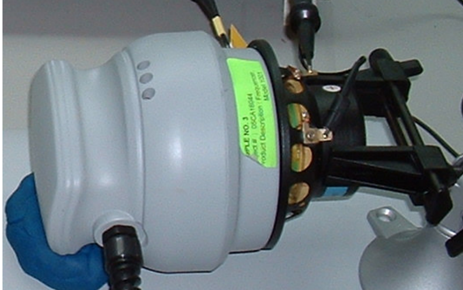
Figure 2: Transducer and loudspeaker setup
